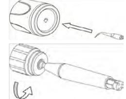
\*To remove sclaer handpiece from tubing, Gently pull straight off. Don't turn / twist or damage to tubing pins will occur.
